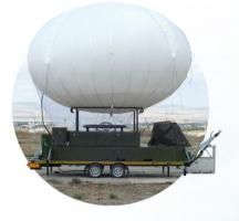
Furthermore, DOLUNAY has a Mobile Anchoring Station that has been designed and produced specifically for the platform, allowing vertical take-off and landing, as well as safe flight and parking.
